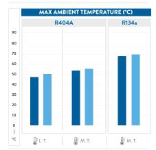
Testing conditions data reference: M.T.: evap. T. -10°C L.T.: evap T. -35°C
