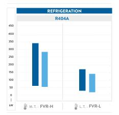
Testing conditions data reference: M.T.: evap. T. -10°C; cond. T. +45°C L.T.: evap. T. -35°C; cond. T. +40°C ECO
