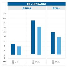
Testing conditions data reference: M.T.: cooling capacity @32°C ambient T.; evap. T. -10°C L.T.: cooling capacity @32°C ambient T.; evap T. -35°C
